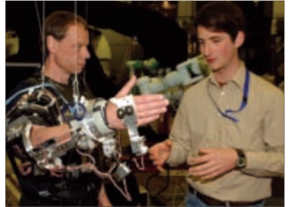
ESA astronaut Christer Fuglesang works with an exoskeleton in the robotics lab at ESTEC. This wearable robot—a combination of arm and glove with electronic aids to reproduce the sensations a human hand would feel—enables a remote operator to work as though he were at a distant site. With haptic telepresence, which adds the sense of touch, anyone purportedly can operate a robot without training. Credit: ESA, J. v. Haarlem.
