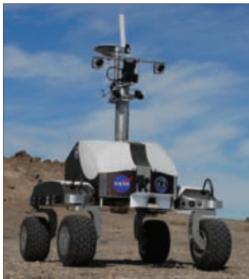
The K10 planetary rover has four-wheel drive and all-wheel steering on a passive rocker suspension, a design that allows operation on moderately rough terrain.
