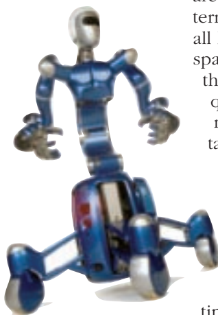
The Justin mobile robotic system was developed at the German Aerospace Center, DLR. With compliant controlled lightweight arms and two four-fingered hands, Justin is an ideal experimental platform. Credit: DLR.
