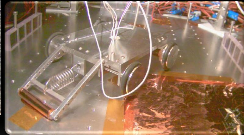
Rolling out Kapton film inside vacuum chamber with teleoperated mini-rover
