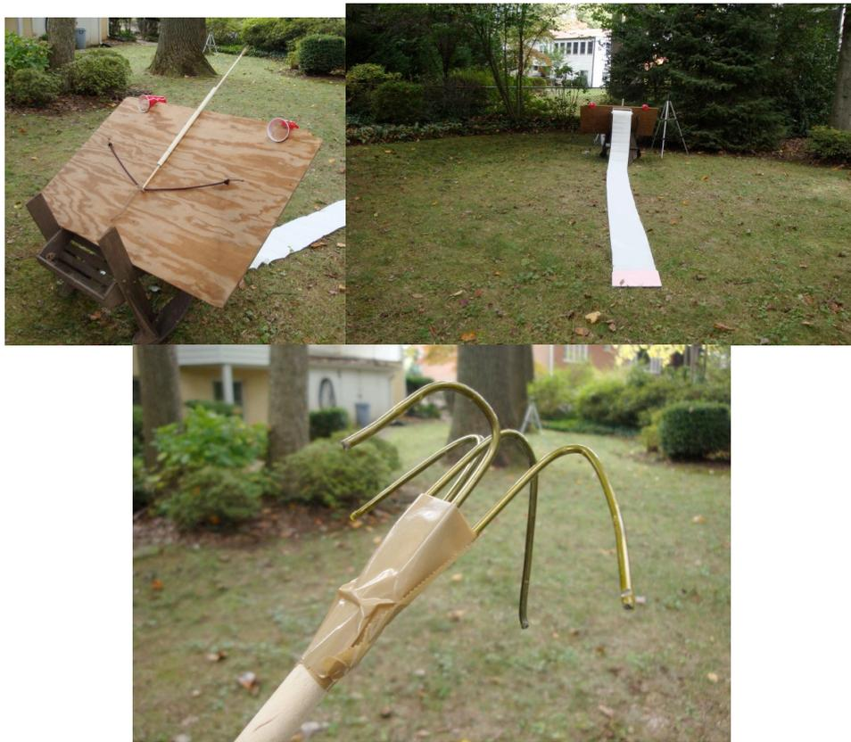
**Figures 33-35:** (upper-left) shows the launching platform. (upper-right) show the deployment of the array. (bottom) show the anchor itself.
