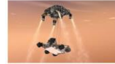
3 Rockets slow spacecraft to halt; "sky crane" tethers lowers rover to surface.
