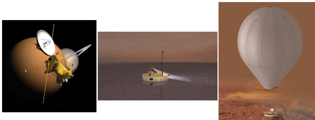
FIGURE 8.13 The three elements of the 2009 TSSM mission architecture: a Titan orbiter, a lake lander, and a hot-air balloon. SOURCE: ESA/NASA.
