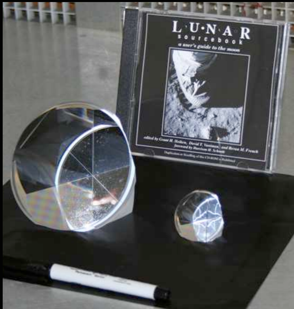
Apollo 3.8cm retroreflector (right), and a 10cm retroreflector just qualified for lunar environment (left)
