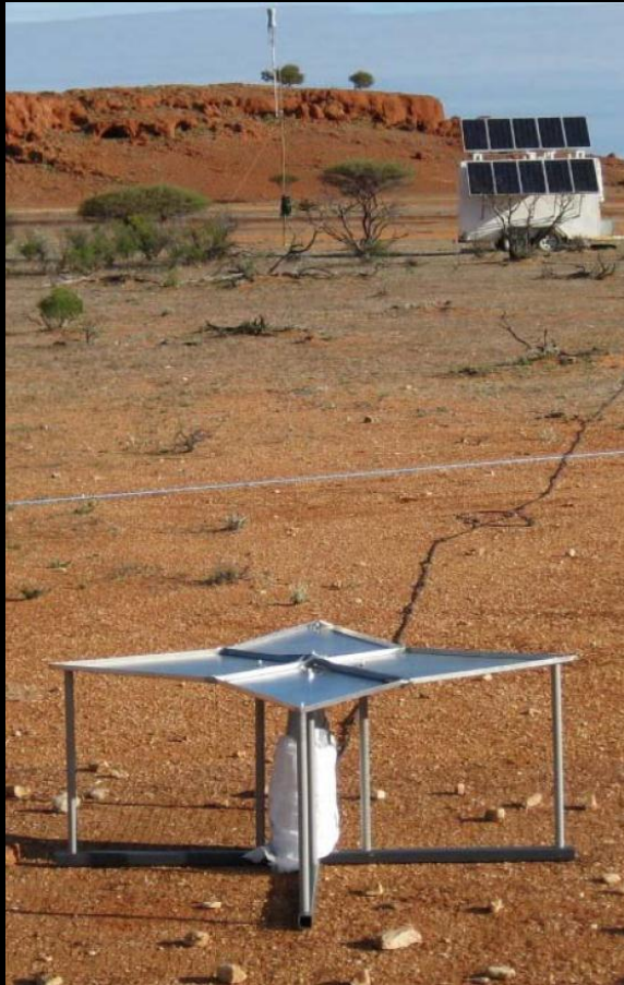
EDGES dipole at MWA site in Western Australia
