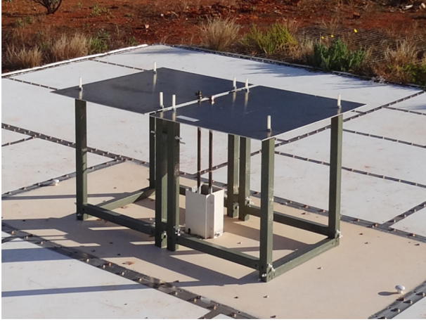
Figure 1. Left: photograph of the high-band blade antenna with fiberglass support tubes and a tuning capacitor on the top of the panels between the balun tubes to improve impedance matching. Surrounding the balun tubes at the base, a short rectangular enclosure shields against vertical currents in the tubes.
