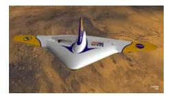
Image Above: Computer-aided-design (CAD) image of the Matador Mars airplane concept. Image credit: NASA Ames Research Center/Andy Gonzalez
