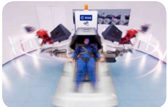
The short arm human centrifuge at DLR enables hypergravity research to understand the gravity impacts on the human physiology and performance.
