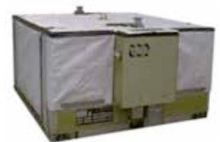
Advanced ISS batteries.
