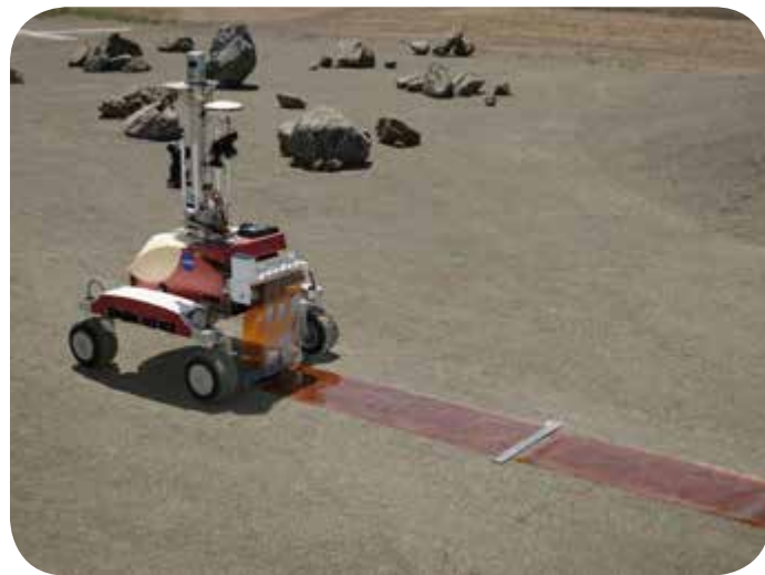
From the ISS, astronaut Chris Cassidy operated this high-fidelity planetary rover, located at Ames Research Center's analogue facility. The ISS is conducting demonstrations such as this to gather engineering data useful to advancing the concept of tele-presence.
