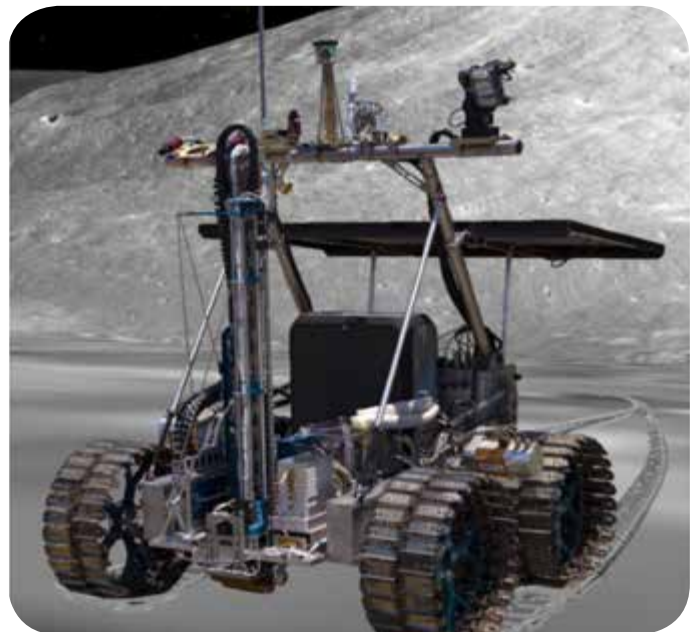
The RESOLVE payload concept shown prospecting for volatiles in a polar region of the Moon.
