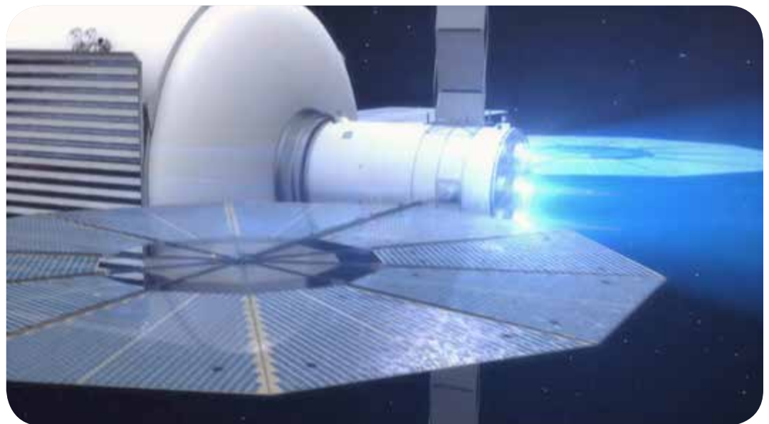
Very large solar arrays with roughly twice the power generating potential of today's state-of-the-art will be needed to power the proposed solar electric propulsion system.
