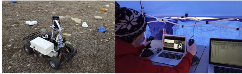
Fig. 4. Left: The University of Colorado student-built, teleoperated rover and exploration targets (painted stones). Right: Operator controlling the rover joysticks ensuring exploration through the rover's twin cameras.
