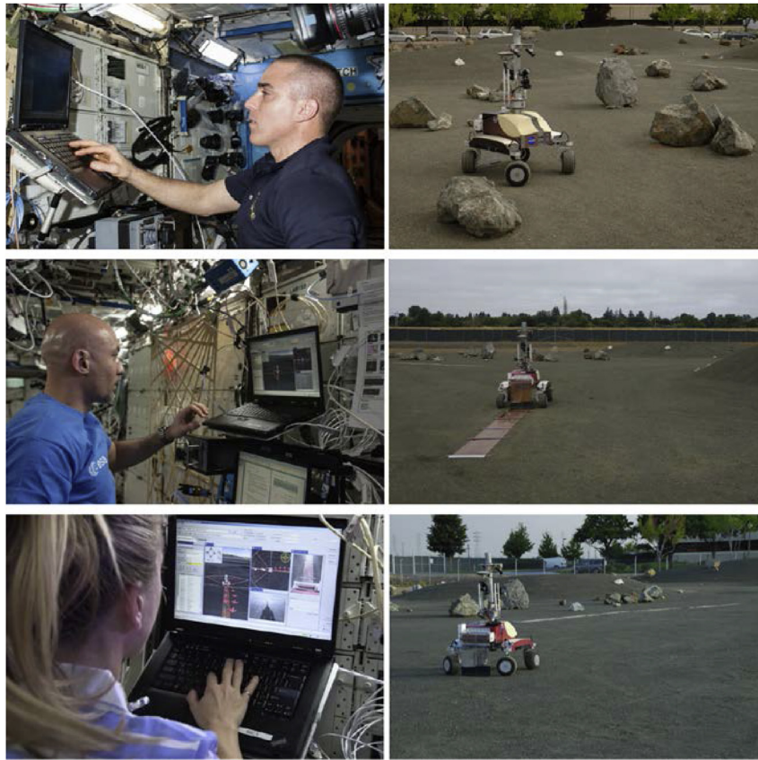
Fig. 3. Surface Telerobotics testing. Top: site survey of the Roverscape at NASA Ames; Middle: deploying a simulated lunar telescope antenna; Bottom: documenting the deployed antenna.
