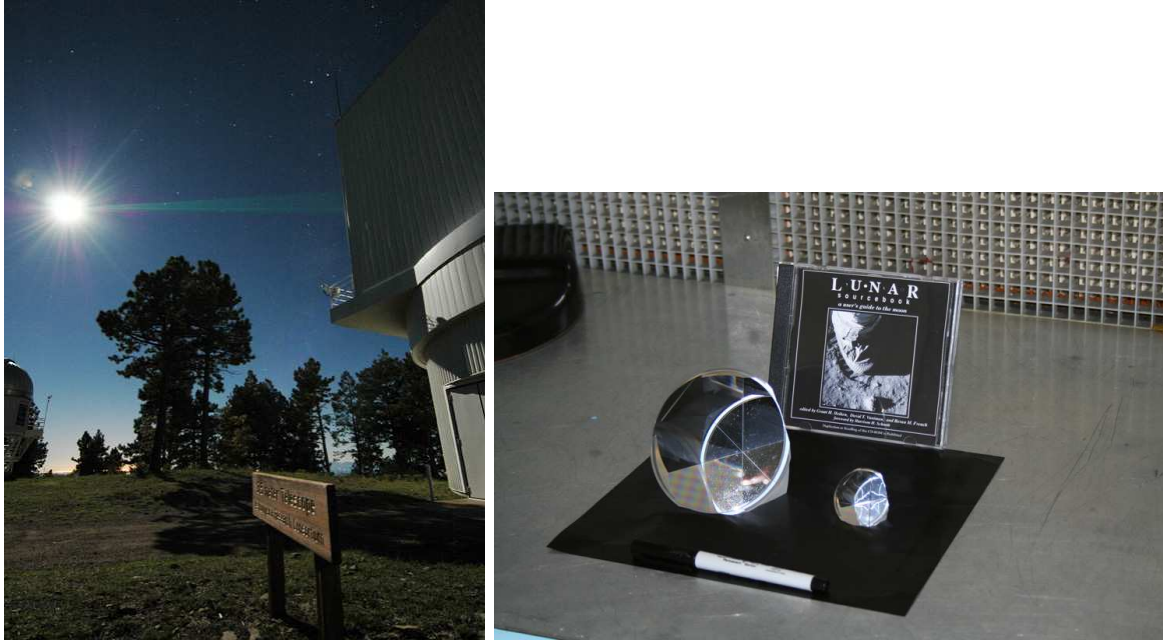
Figure 10: Left: APOLLO LLR shooting the Moon from Apache Point, NM. Right: Prototype 100 mm next-generation corner cube next to a 38 mm Apollo engineering model corner cube.
