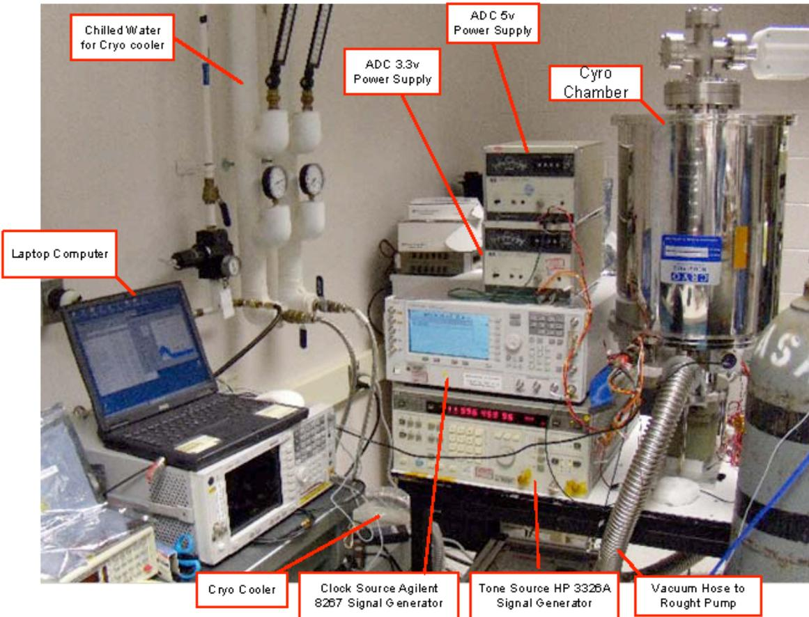
**Figure 29:** Show the testing of the analog to digital converters needed for a lunar low frequency radio array.
