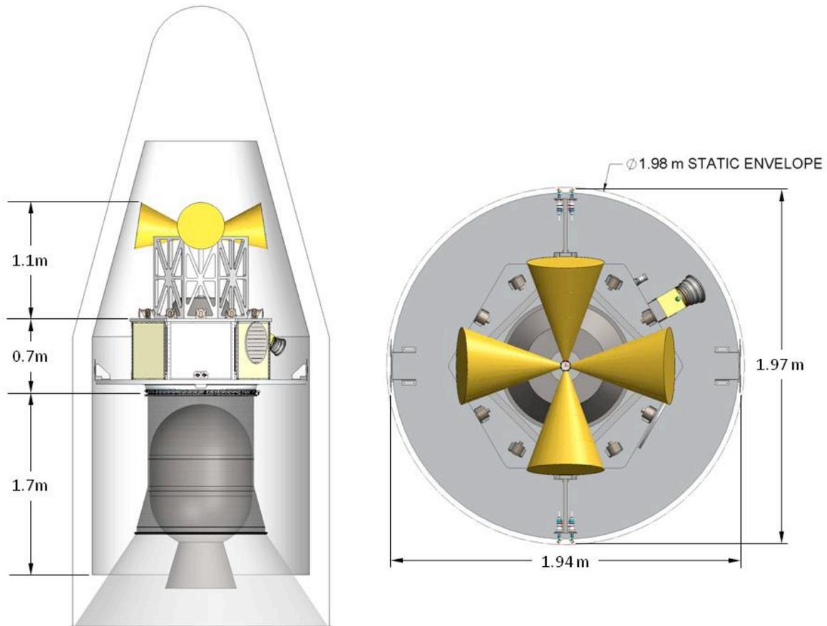
**Figure 17:** (left) Shows DARE's launch configuration inside the faring of its launch vehicle and the instrument layout (right).
