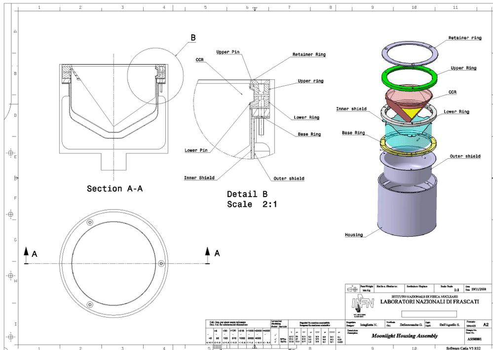
**Figure 42:** Shows more of the design specifications for the LLRRA 21 package.
