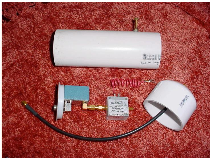
*Figure 13: A low noise amplifier and a 50-to-75 W transformer were mounted inside of a weather-proof enclosure and connected to the antenna terminals from beneath the ground plane.*
