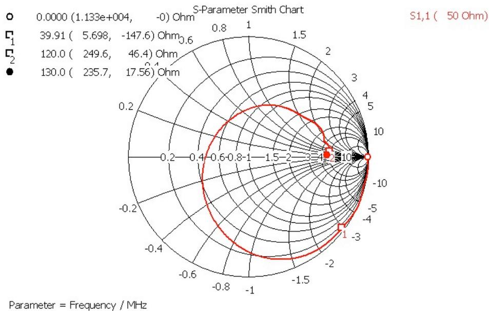
**Figure 20:** Shows the terminal impedance as a function of frequency plotted on a Smith Chart.
