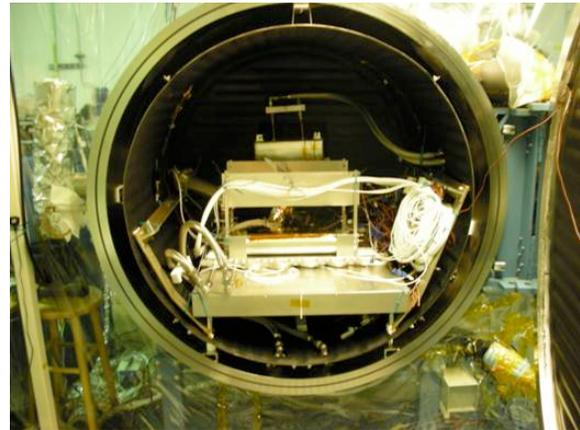
*Figures 15 & 16: (left) shows some of our undergraduate and graduate students working on our experiments outside the vacuum chamber. (right) shows the experiment inside the vacuum chamber prior to simulating the lunar environment.*
