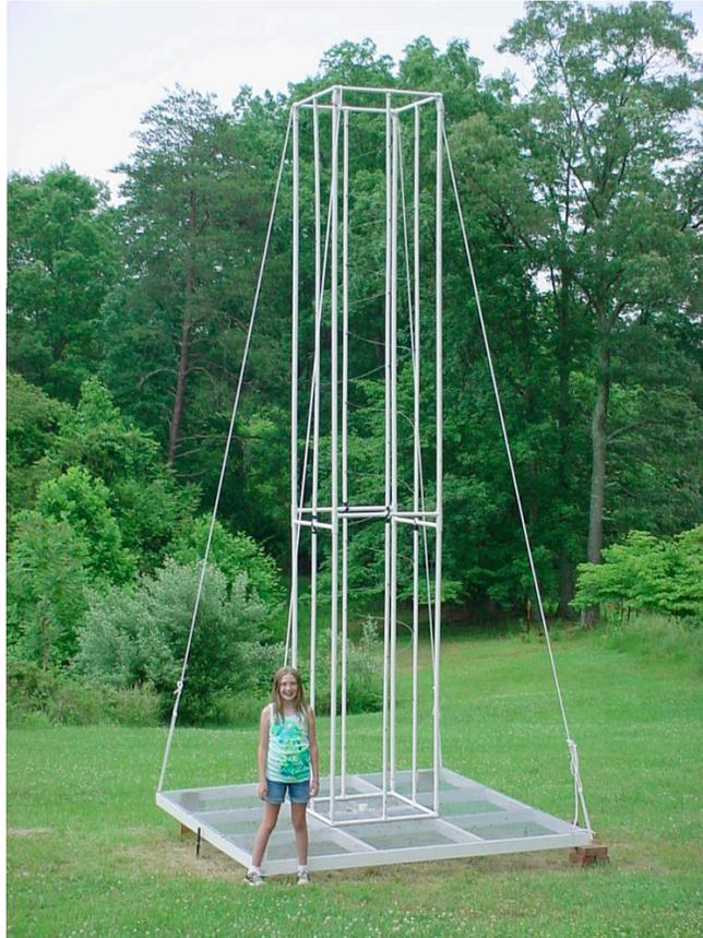
*Figure 12: The antenna was constructed using #18 gauge copper wire supported by a dielectric framework of PVC tubing.*
