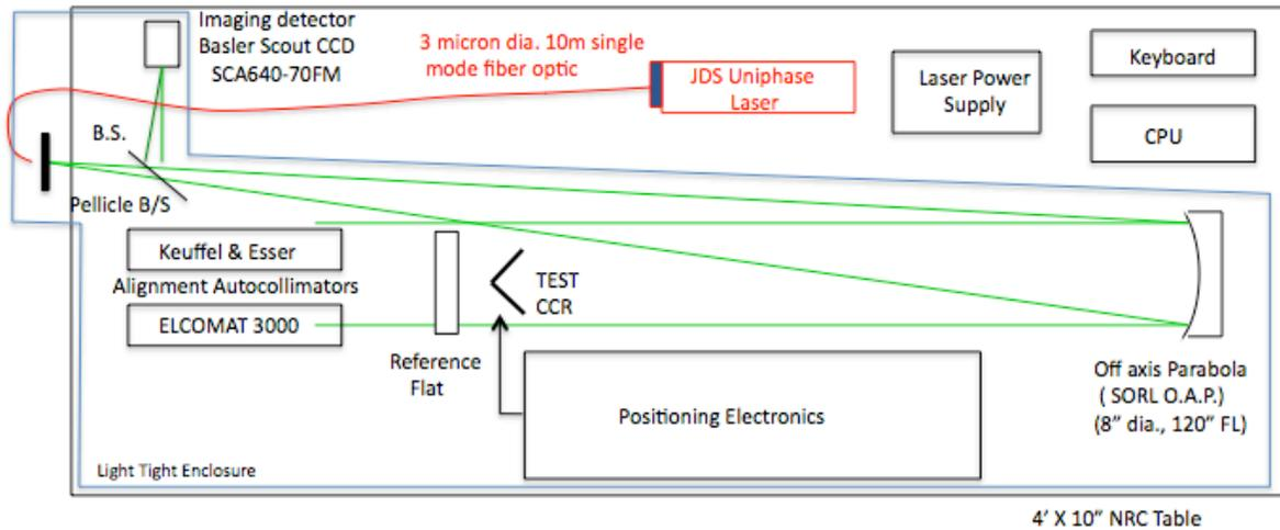
*Figure 37: is a simplified block diagram of the cube corner test setup.*
