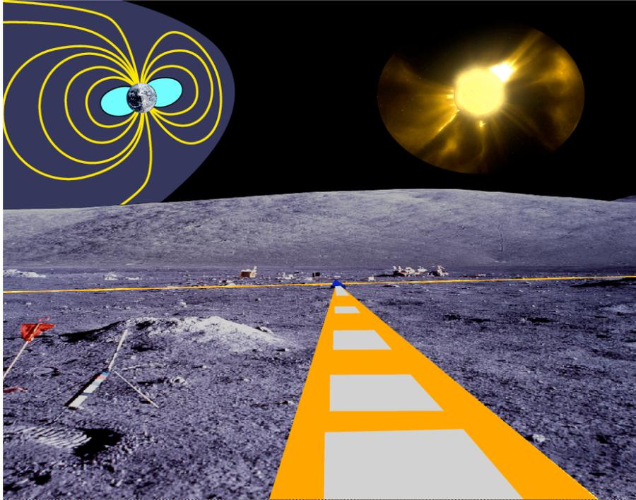
**Figure 3:** This show the ROLSS concept (Radio Observatory on the Lunar Surface for Solar studies). This array would be comprises of single radio dipoles embedded within polyimide kapton film.
