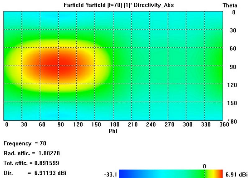
**Figure 19:** Shows a typical beam pattern of the DARE instrument.
