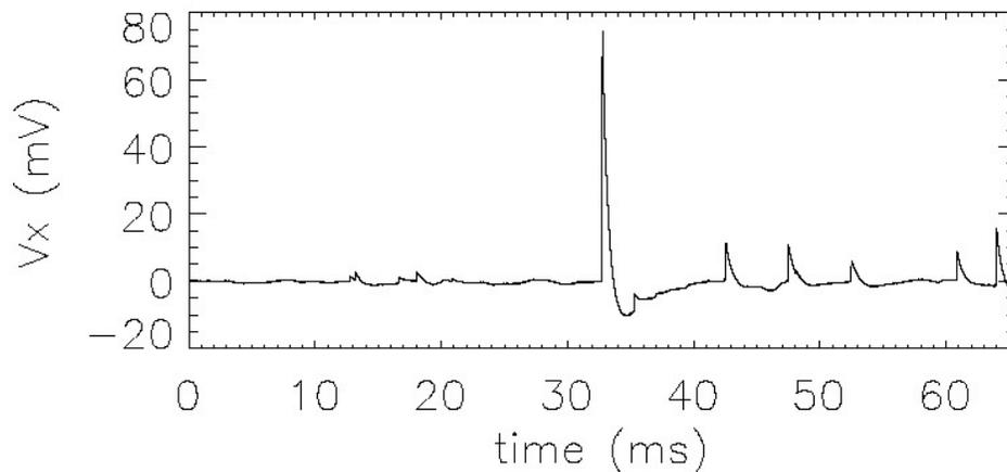
**Figure 22:** Shows data of dust impacts measured from the WAVES instrument onboard the STEREO A & B spacecraft.
