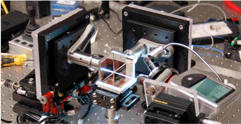
**Figure 4:** This is one of our next generations of Corner Cube Reflectors CCR to help constrain our distance measurements from the Earth to the Moon.
