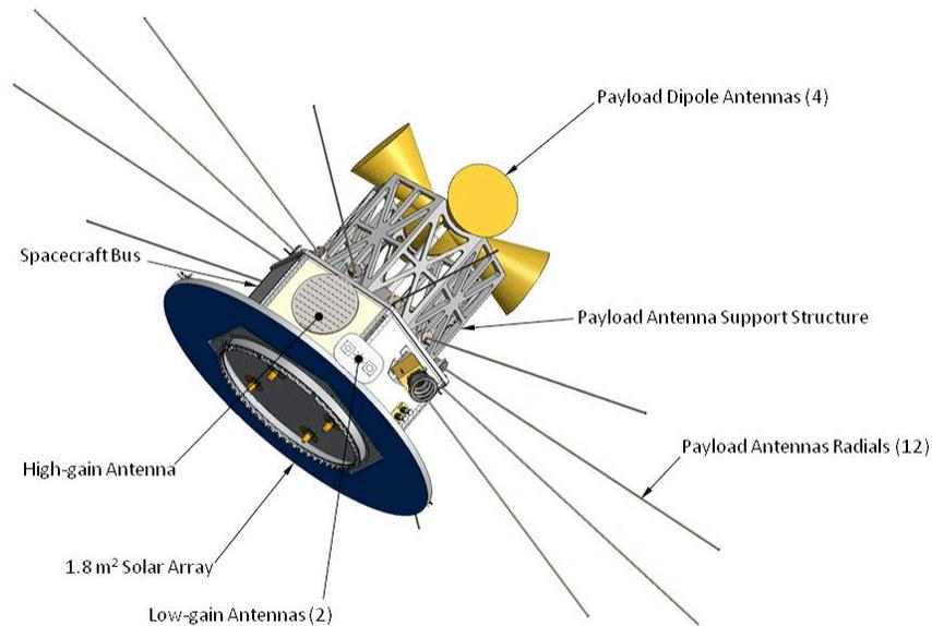
**Figure 18:** This shows DARE in its operational configuration.
