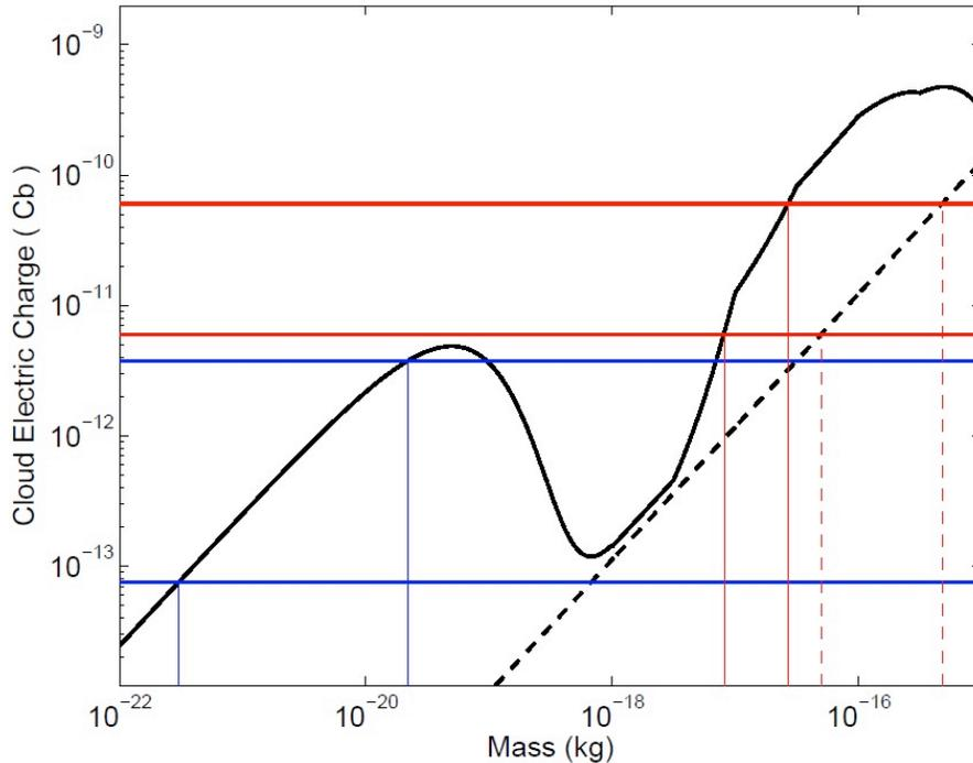
**Figure 23:** illustrates our mapping between freed charge and initial dust particle mass for the STEREO spacecraft.
