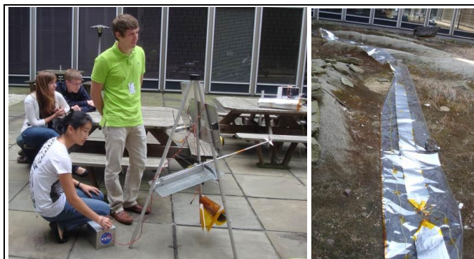
Fig. 6. (Left) GSFC summer interns with cross bow-launched anchor deployer. (Right) Inflatable tube with dipole antennas; the tube has been deflated after a successful deploy.
