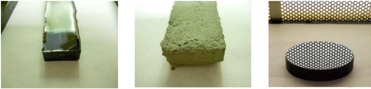
*Left & Center:* Samples of ‘lunar cement’ made with lunar regolith simulant and epoxy at different proportions. The ratio of simulant to epoxy that could make a robust material turned out to be quite narrow. On the left is a 3:1 sample. At 5:1 (center), the material was crumbly and had very low structural strength. *Right:* A 5 cm diameter lunar cement disk was polished into an optical flat. The experiment suggests that future telescopes on the Moon can be made in-situ using lunar dust.
