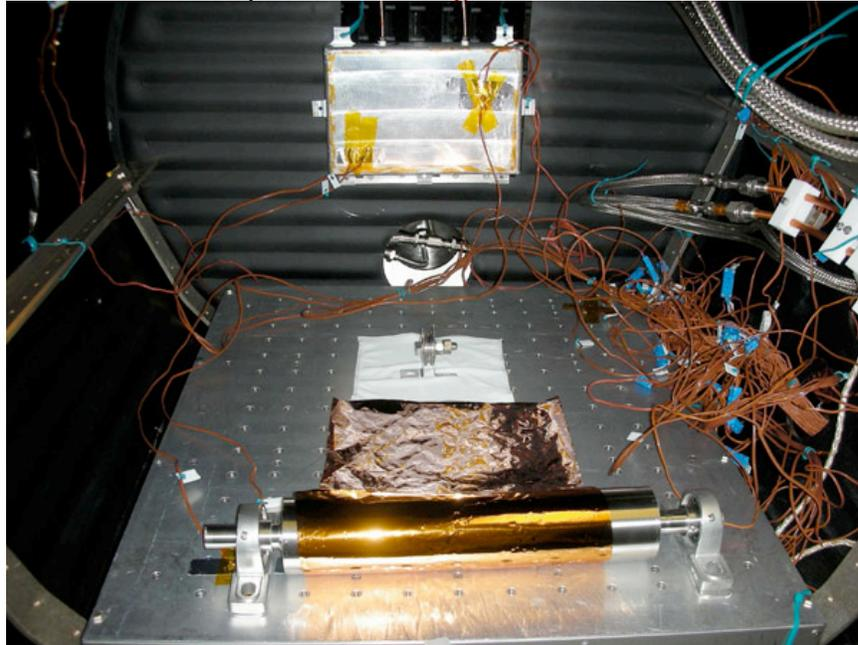
Figure ES 2: Testing of polyimide film in a vacuum chamber at the University of Colorado
