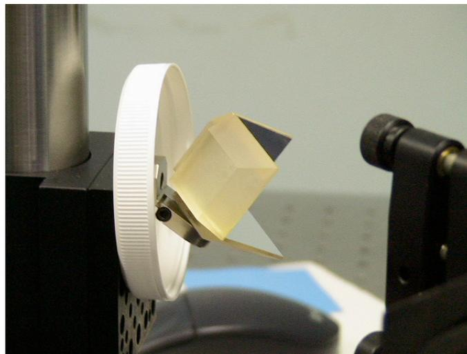
**Figure RH 3:** PLX 1.5" diameter zerodur cube corner
