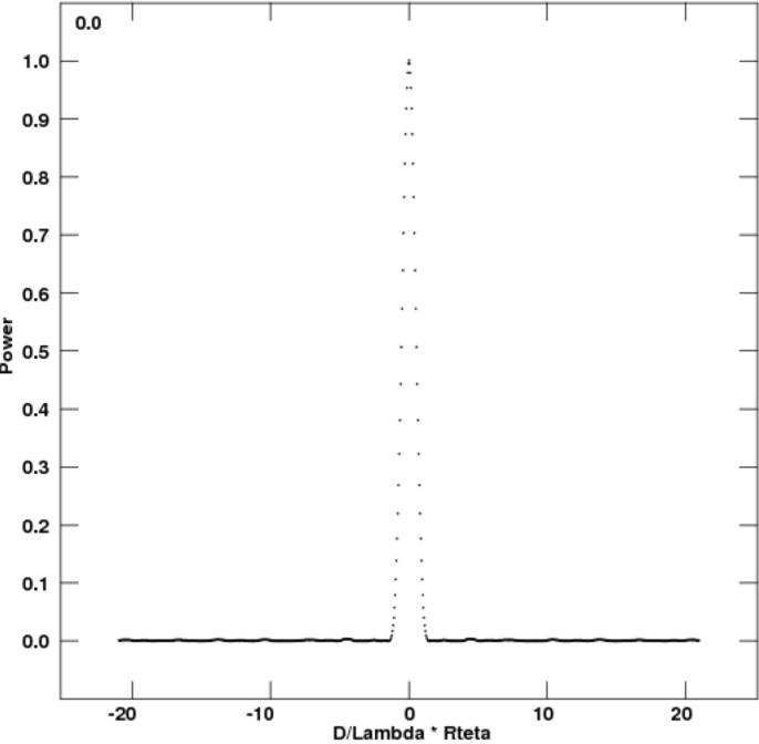
Fig. 4.— Beam pattern for the 459 element configuration shown in Fig. 3.
