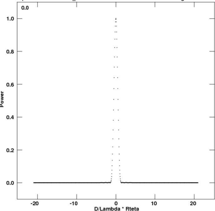
Fig. 6.— Beam pattern for the 828 element configuration shown in Fig. 5.
