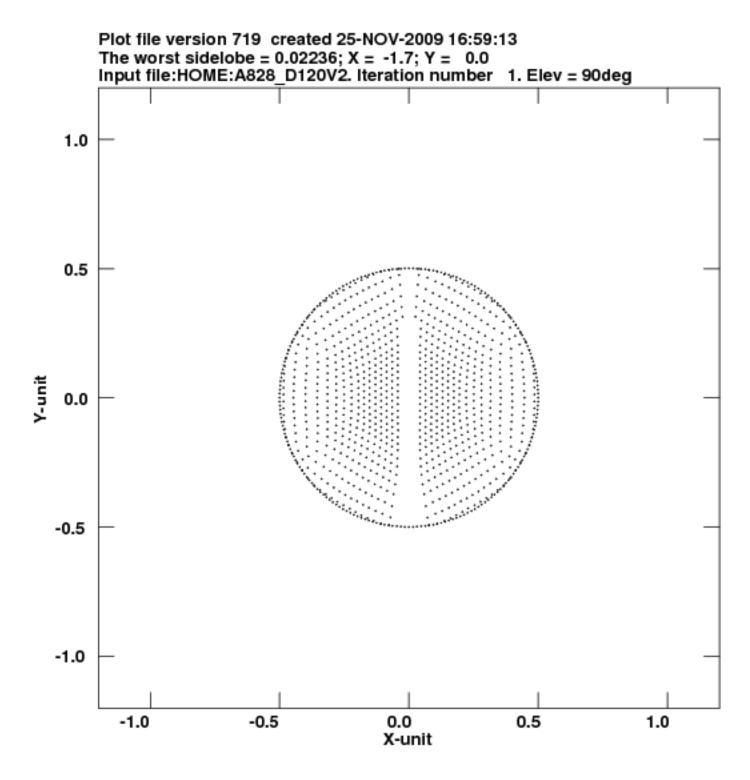
Fig. 5.— Optimized hexagonal station configuration after the systematic failure of 10% of the elements.
