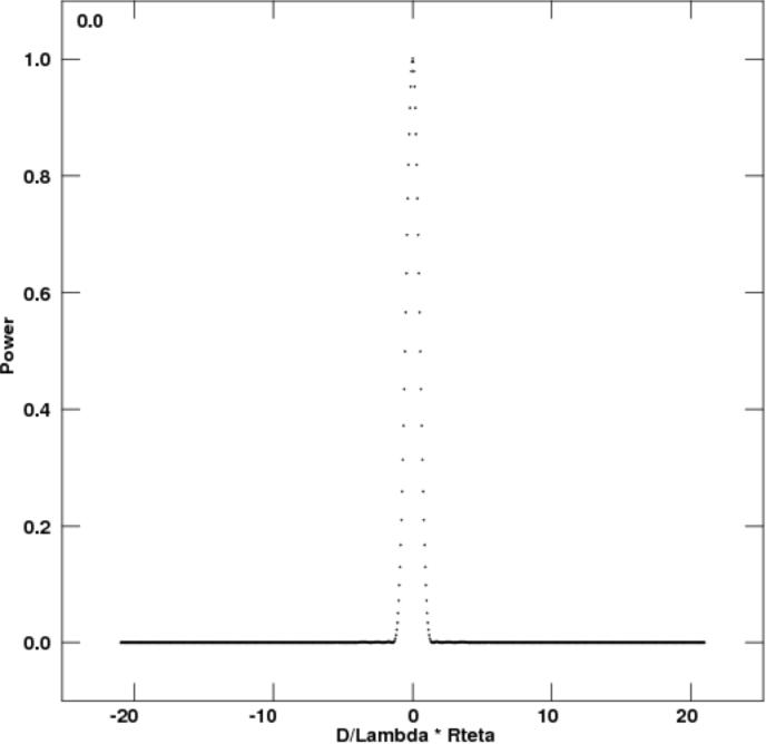
Fig. 2.— Beam pattern for the optimized 919 element configuration shown in Fig. 1.
