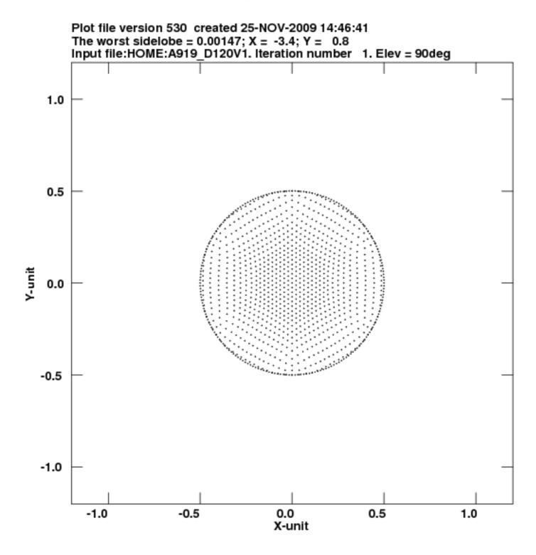
Fig. 1.— Optimized hexagonal station configuration used as a starting point for the analysis. There are 919 antennas inside a circle of diameter 120 m. A minimum spacing of 3 m between the elements was used.
