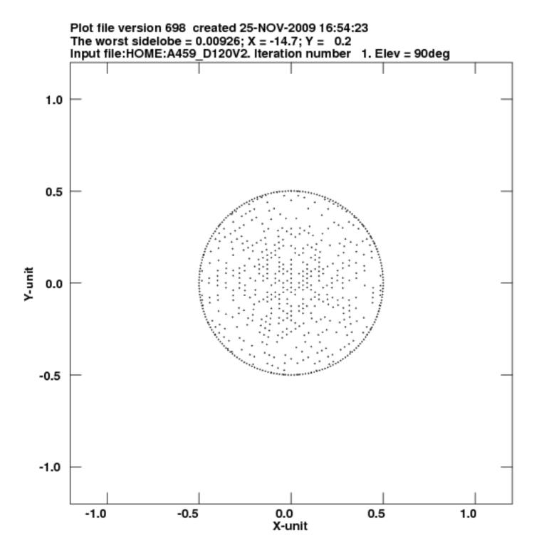
Fig. 3.— Optimized hexagonal station configuration after the random failure of 50% of the elements.
