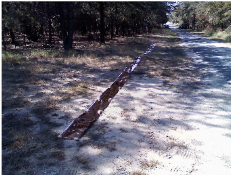
Figure 2: The antenna was tested in two positions: (1) on sandy, partially grass-covered soil (as shown), and (2) on an asphalt road (visible on the right side of the picture).
