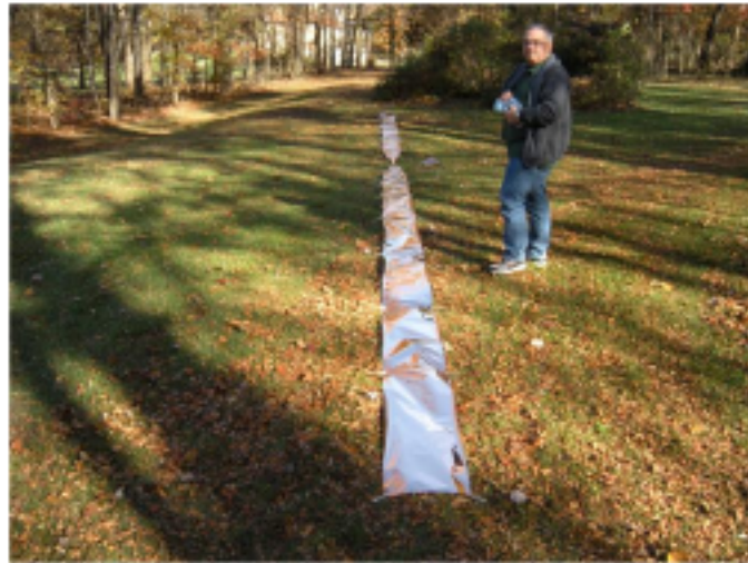
Figure 1: The polyimide film antenna as deployed. The antenna was tested on moist, grass-covered soil.
