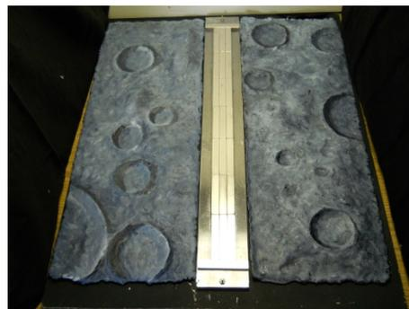
**Figure 17.** A model to demonstrate a lunar space launch system made using superconductors and lunar cement.
