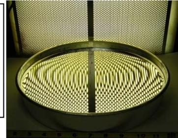
**Figure 15.** A prototype 'moondust telescope mirror' made with lunar cement.
