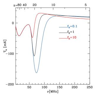
**Fig. 2.** Brightness temperature of the hyperfine transition of the ground state of atomic hydrogen (the wavelength of this transition is 21 cm), averaged over the entire sky, as a function of redshift z for the same three different values of  $f_X$  as in Fig. 1.
